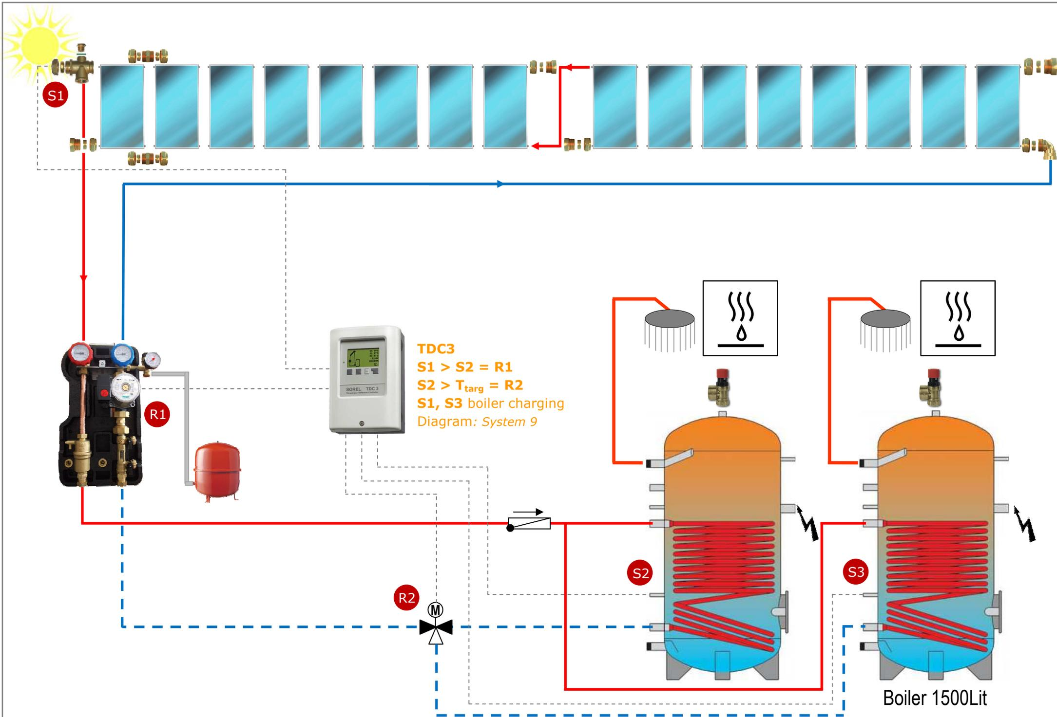
**Hydraulic diagram:** 2 storage tanks, internal heat exchanger, pump and valve logic
